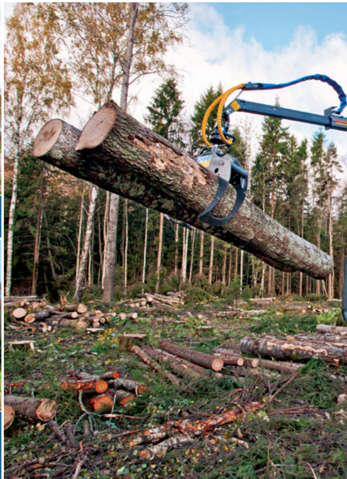
The picture shows the C 5.3 G2 mounted on a 9-ton trailer. The trailer is additionally equipped with "lightweight valve", crane lighting and radio controlled winch.
