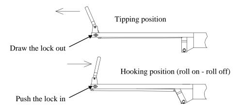
**Note!** The bolt needs to be locked within the handles extreme position *Figure 32. Changing operating function*
