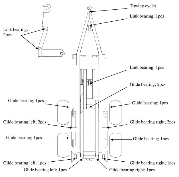
Figure 38. Lubrication points
