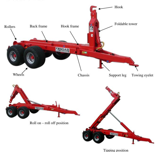
Figure 1. Design of the device
