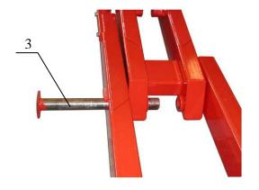
Figure 40. Back and hook frame coupling
