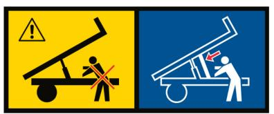
Figure 24. Use the safety support during all service
