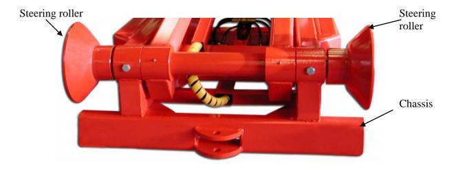
Figure 12. Steering rollers
