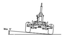
Place the hooklift trailer on a flat surface. The sideways incline may not exceed 5 degrees.
