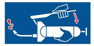
Figure 30. Lubricate points.
