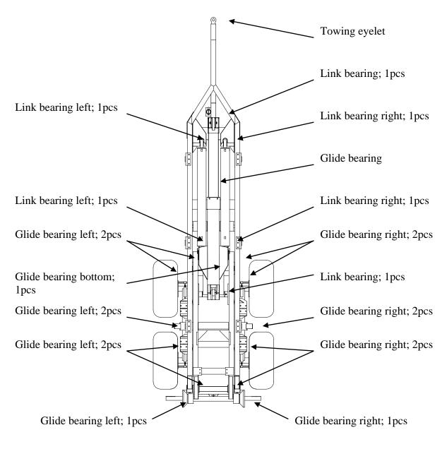
Figure 39. Lubrication points
