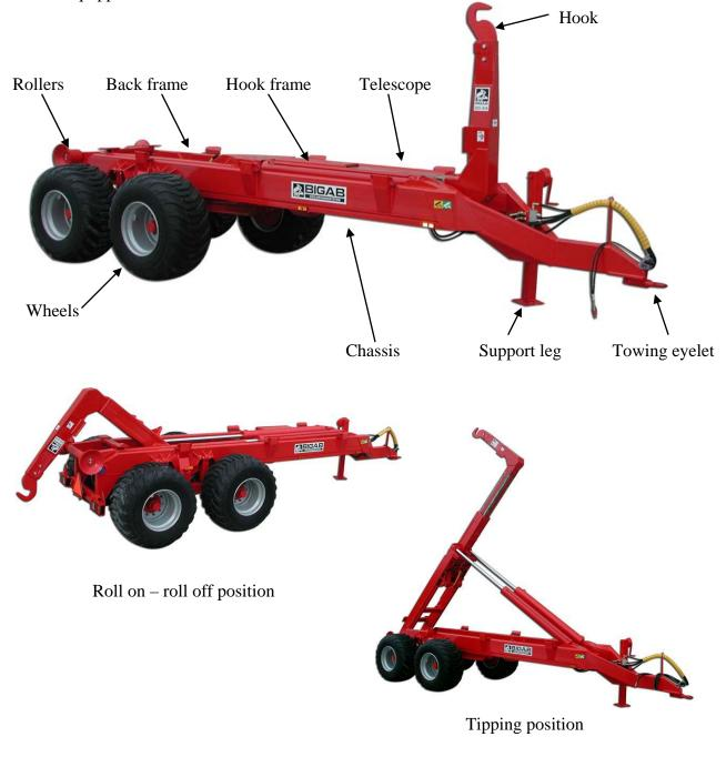
Figure 1. Design of the device
