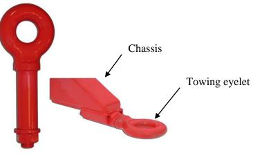
Figure 9. Towing eyelet
