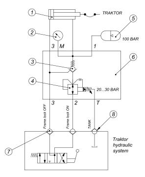
Figure 36. Frame lock hydraulic system.
