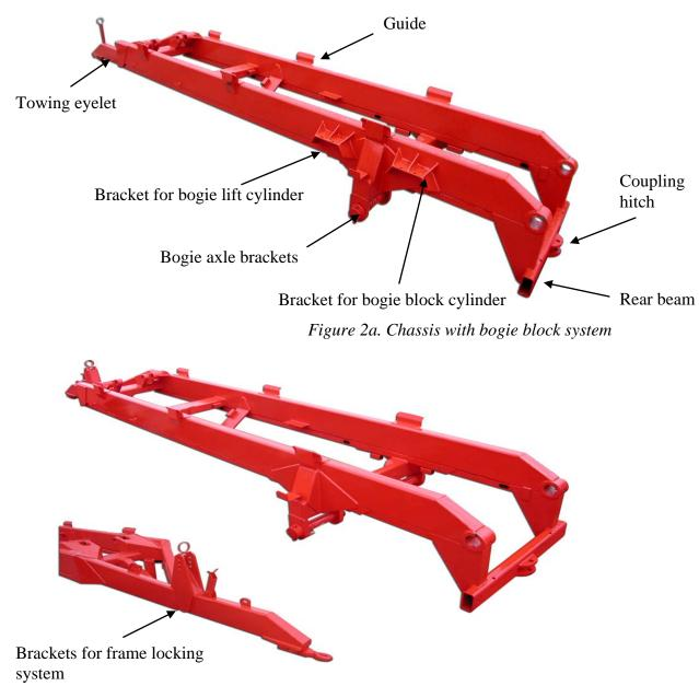
Figure 2b. Chassis with frame locking system
